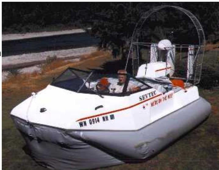
The sev is now sold as plans and kits for a single or two engine craft under the name Surveyor. See Sevttec and follow the Surveyor link. Engine options are a single 25hp Kohler to the Kohler plus a 16hp Vanguard for lift. Other engine combinations may be used. (Note use of the Kohler requires an operational electric system.) Check with Sevttec or [Amphibious Marine](#) for additional information.
