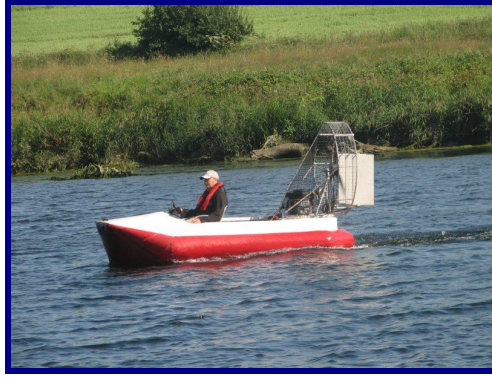
Pic 05-04 A home-built twin fan SevTec Scout. ( http://members.aol.com/sevtec/sev/skmr.html )
