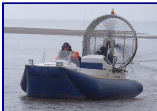
Pic 04-04 SevTec craft fitted with compartmented responsive skirt
