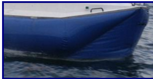
Pic 06-04 A low pressure bag skirt
