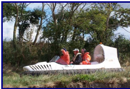
Pic 05-05 A 3 seat twin-engine craft from BBV ( www.bbvhovercraft.co.uk )
