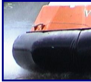
Pic 06-03 A high pressure bag skirt
