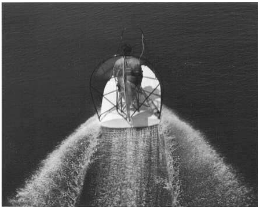
This airboat is powered with a 15 hp JLO L 230 engine.
