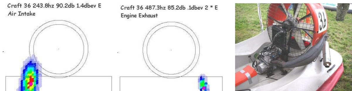
Fig.7. It was expected that the air intake on this craft would be loudest as it has a good exhaust silencer. The crankcase noise however was unusual and reported quickly to the driver. 3 races later it seized.
