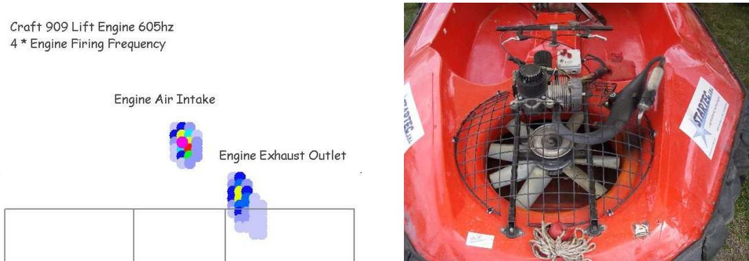
Fig.6. This craft has an engine air intake about 5db louder than the exhaust. It has a good exhaust silencer but doesn't have the airbox intake silencer that is often fitted to snowmobile versions of this engine.
