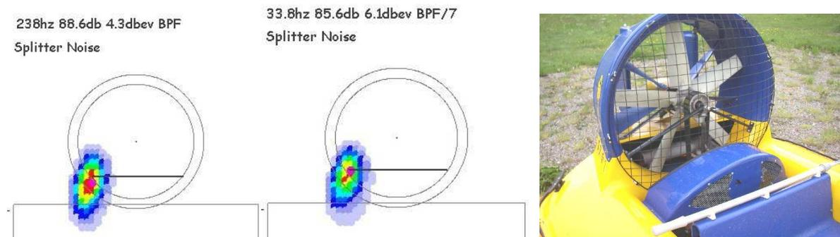
*Fig. 4. Other obstructions close to the fan cause turbulence and thus noise eg an engine pulley 50mm from fan tip and a radiator 150mm away whose turbulence has been displaced by air swirl*
