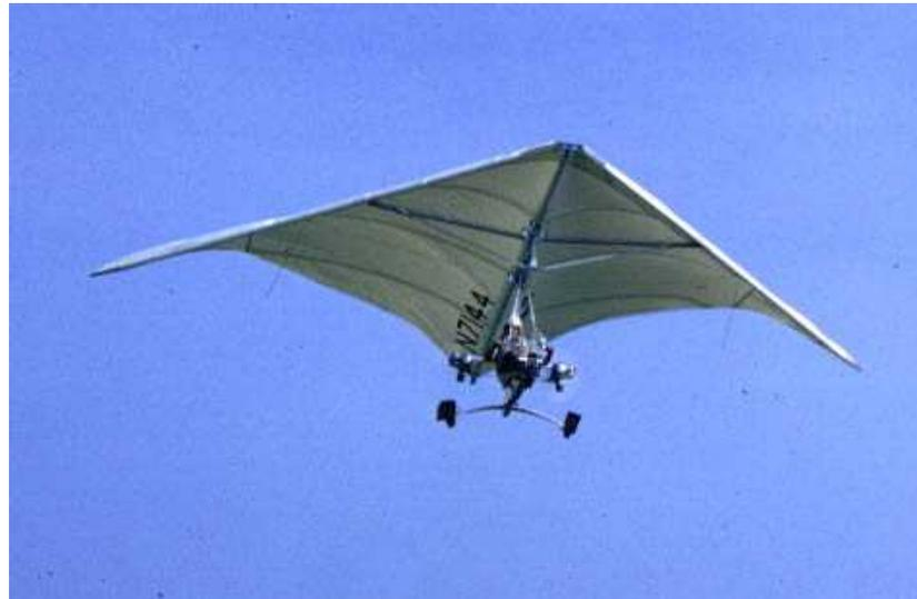
Completed in March of 1967, This is possibly the earliest example of a trike. "Paraplane" used two West Bend (Chrysler) 820 engines (8hp @6000rpm, reduced to 4700rpm maybe 6.5hp for a total of 13hp, for propeller matching reasons) direct driving a pair of two blade 27in diameter polyester fiberglass over balsa propellers. The craft took off, flew, and landed at very near to 25mph.
