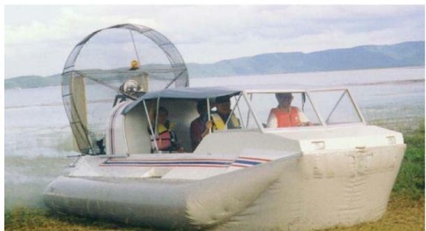
neater, and **cruising comfort** may be had. With a hull size of 8 feet by 16 feet or the preferred 18 feet, Prospector is a scaleup of the Vanguard design, and uses a Subaru 1.8L EA82 engine. Prospector uses a drive similar to the North to Alaska Explorer.
