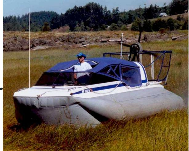
With a hull size of 8 feet by 18 1/2 or 20 feet, Explorer is a scaleup of the Vanguard design, and uses a Subaru 1.8L EA 82 engine. Two aluminum frames automatically extend when the engine is started so this sev flies as if it were ten feet wide. (Note! The drawing shows the sev at flight configuration, 10 feet wide to the edges of the aluminum frames. It does automatically fold for highway trailering under 8 ft width.)
